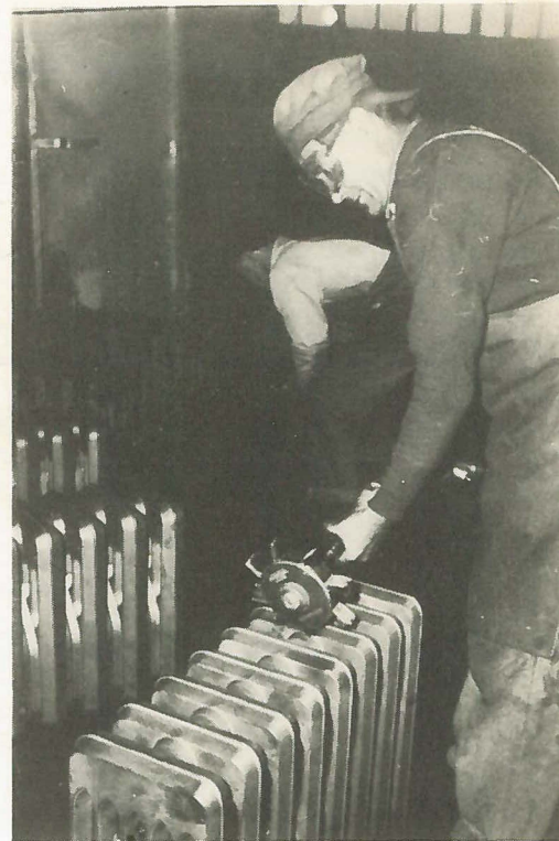
Jesse Wiandt, Gasteam Assembly, using the new Sand-O-Flex polishing wheel which was purchased to smooth the tops of our radiators before painting. This tool does a better job than filing and is less fatiguing to the operator.
