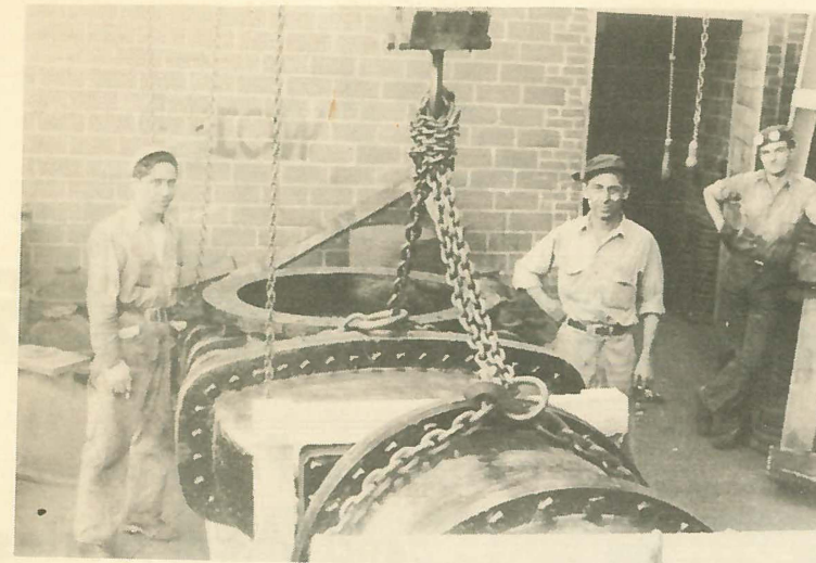
Max Jackson (l.) and George Young stand beside one of our 36" hydraulic valves. This one weighed approximately 8 tons and is the first of an order for that size.
