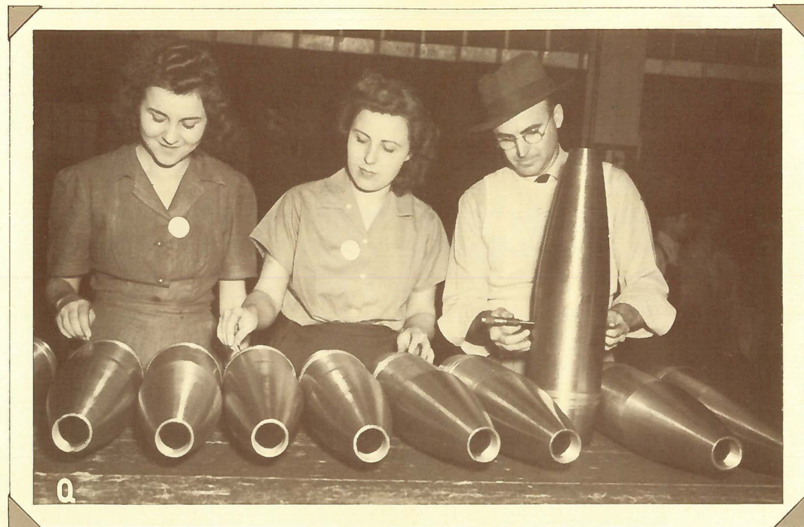
Inspecting and gauging finished metal forms for 155 millimeter shells, Birmingham plant
