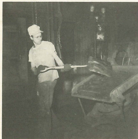
Jack Vanve of our shakeout crew riddling sand on the crane floor. Jack does a fine job and seems to enjoy his work.
