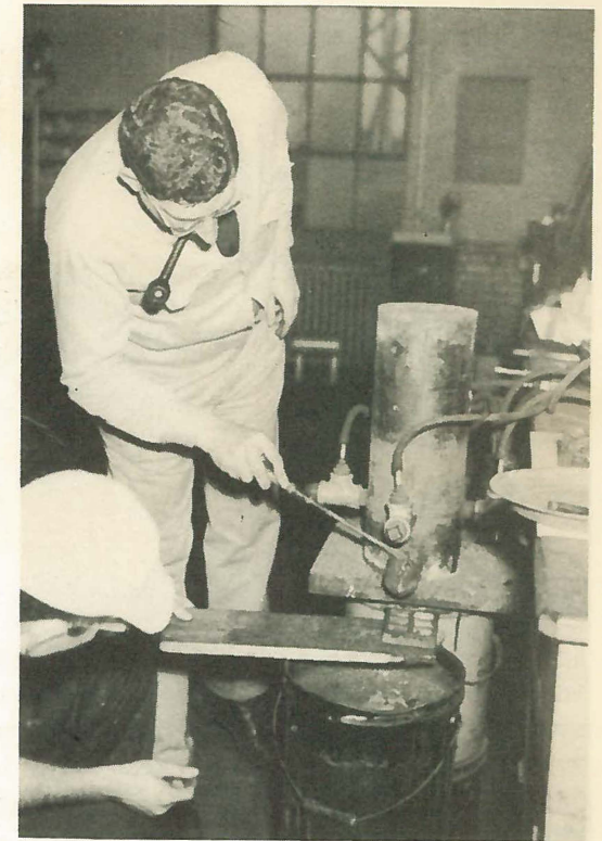
M. D. Neptune and Tom Reese are shown operating the miniature cupola that is used in the Laboratory for experimental purposes.
