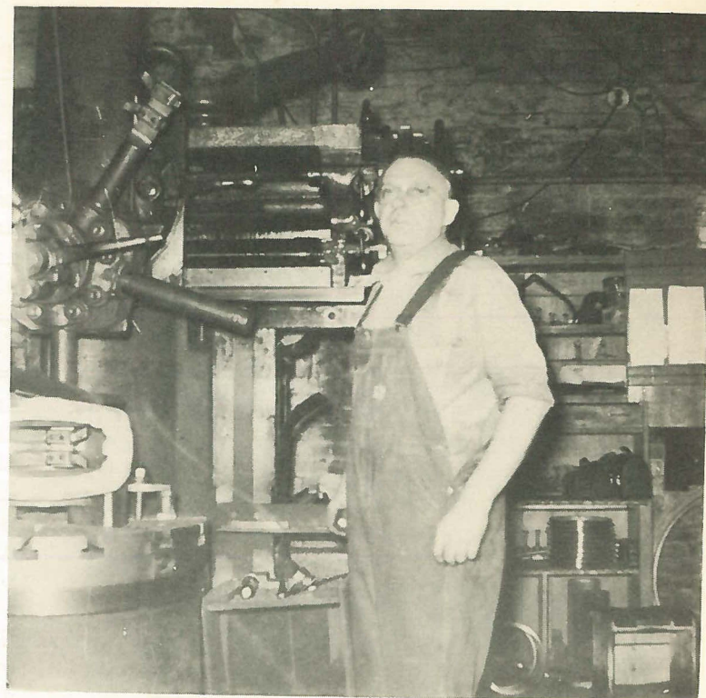
John Van Ee seems serious as we interrupt his valve ringing work. John and his Bullard vertical lathe function with the ease of a single machine.
