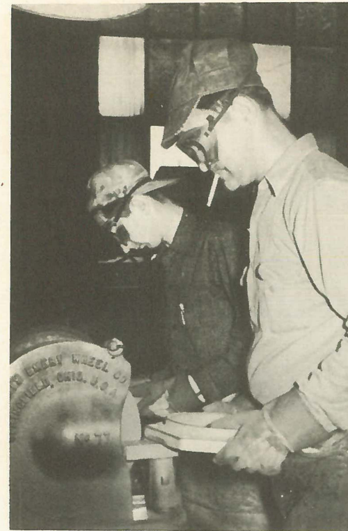
Grinding glands in the Finishing Department - Carl Blizzard (foreground) and Robert Lorenz.
