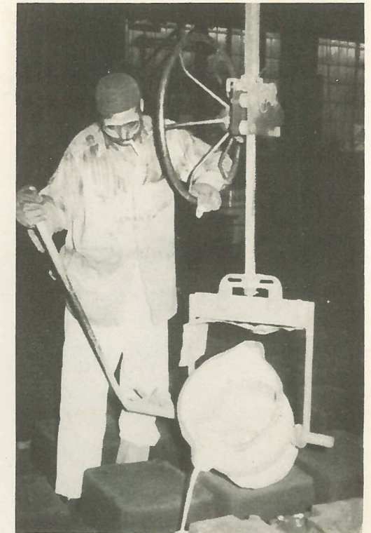
Iron is poured into one of the many molds laid down daily by Ed McCall.
