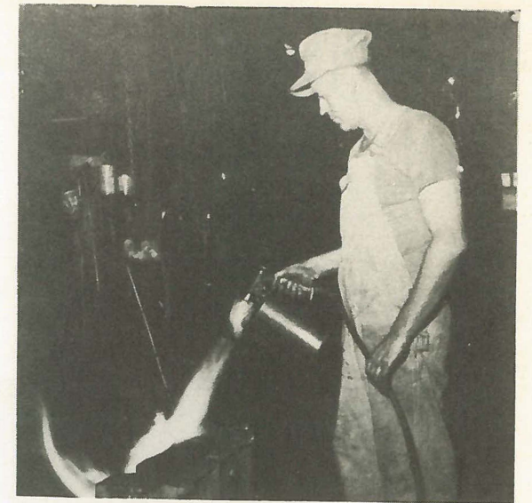
In this picture, Archie Braden - crane floor molder - was drying one of his molds with an oil fired torch.
