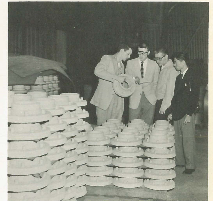
RALPH REID, left, is shown explaining cores used in the manufacture of cast iron pipe.
