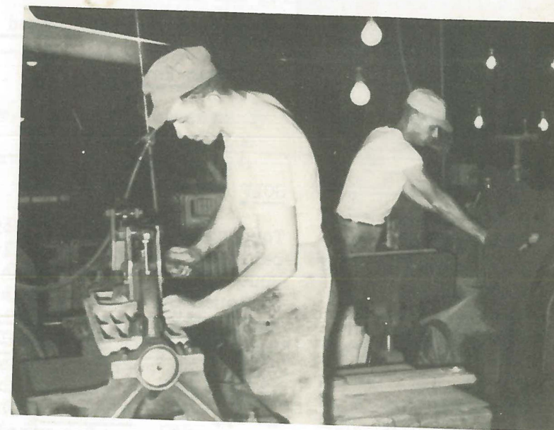
Willard Donley, on left, water testing radiator loops. Sam Gibson, on right, reaming radiator loops. Willard was a suggestion winner in the month of May.
