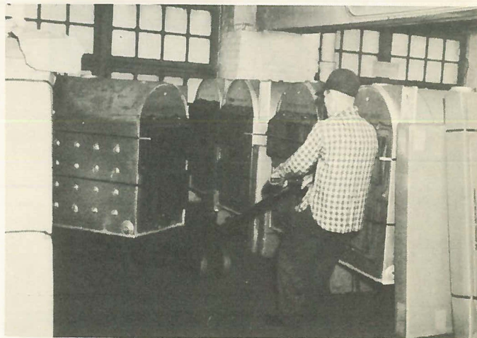
JACK LIFT trucks provide one-man handling of steel boilers stored on platform.
