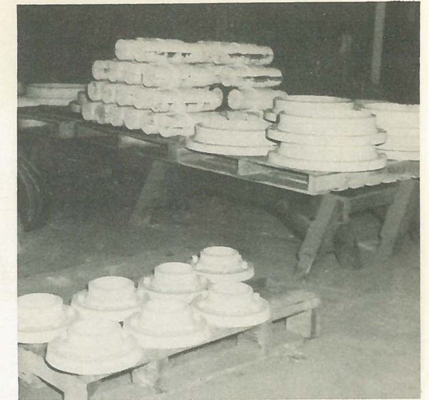
Above are some of the first cores that were made and treated through the new dielectric oven in the Specials Foundry.
