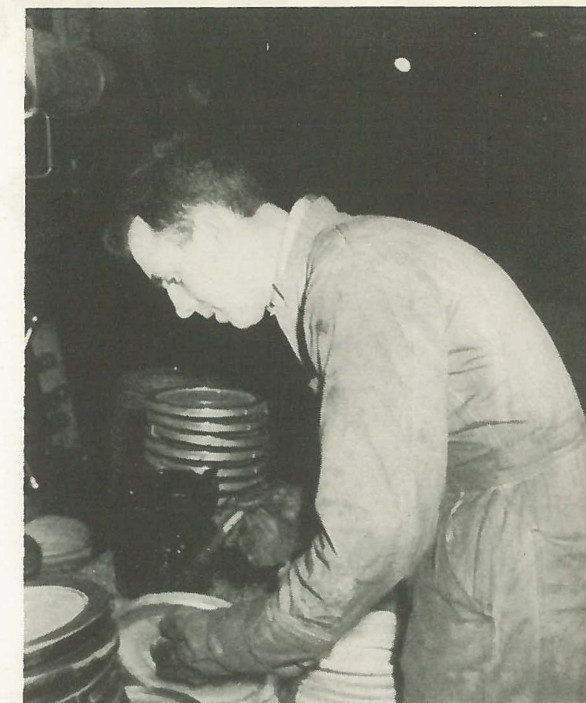
Scotty Scullon is shown above putting a coat of paint on some of our 6-inch Eddy gates.
