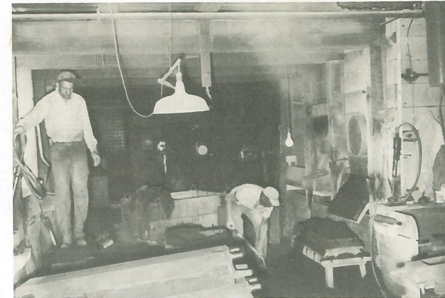
Tom Coker, on left, and Elton Collins, at work making a 6-32 inch loop mold.
