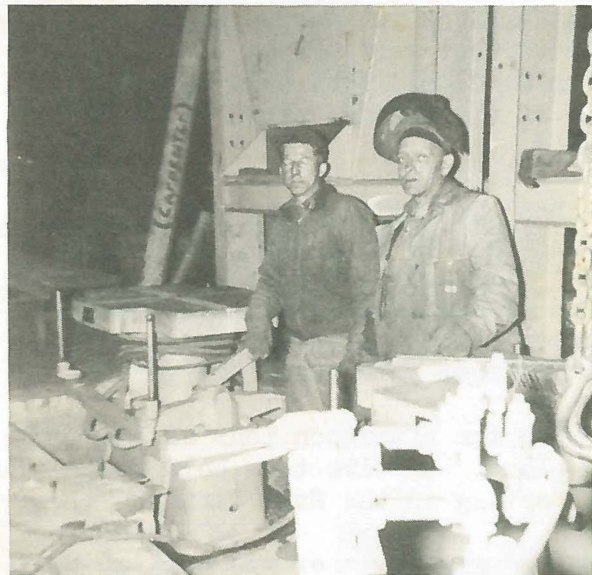
Vernon Peck and Ernest Tidrick installing the new jolt pin lift molding machines.
