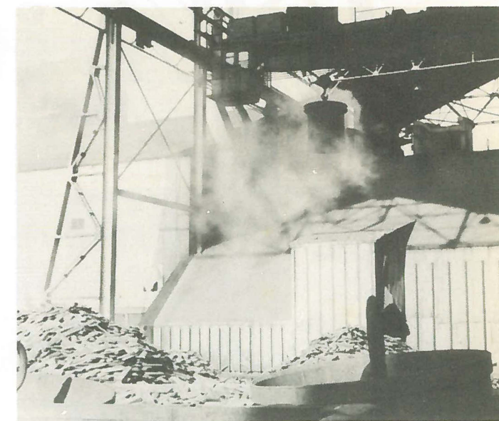
A view of the charging crane lifting the charging bucket to the top of the cupola.
