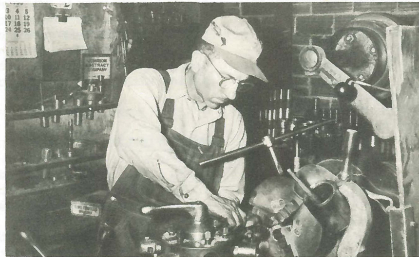
Bill Fisher carefully sets the tool on his small brass lathe preparatory to starting a new job. Bill was recently moved to this new location.
