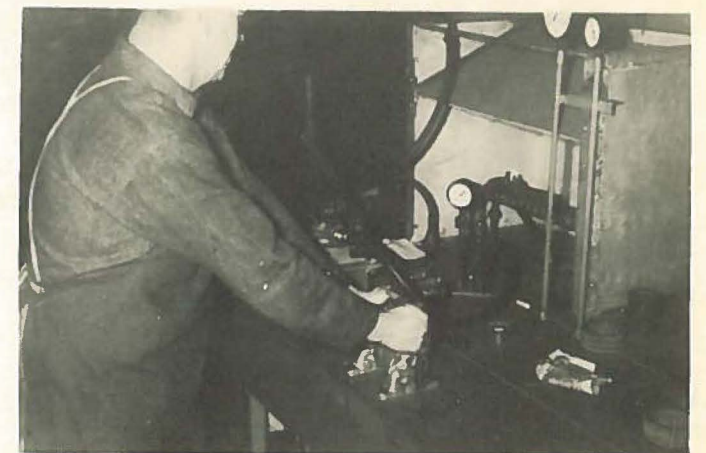
Ben Hartline tests Gasteam pressure regulators on the new test bench which was installed in our Gasteam Assembly several months ago.
