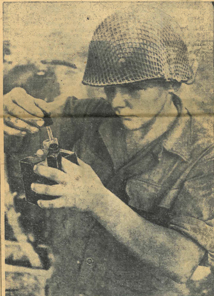
A POCKET CHEMICAL KIT is used by an American soldier to check on the purity of water pumped from a stream in Italy. A U.S. division requires about 50,000 gallons of water a day.
