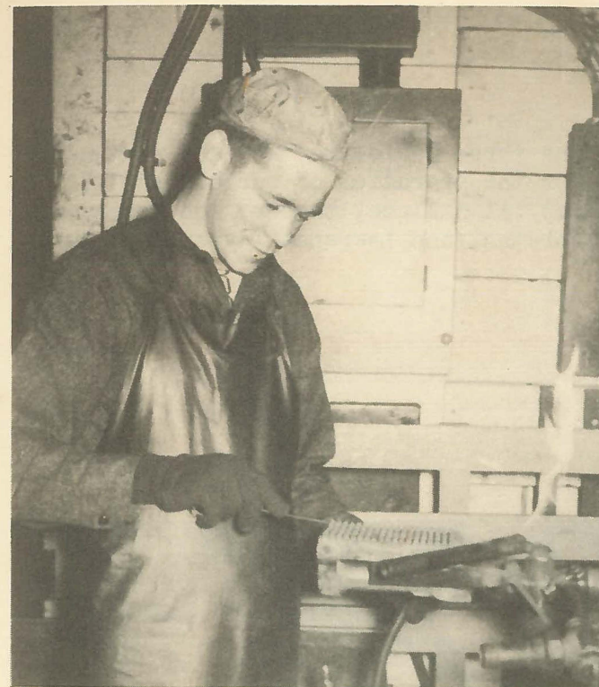
James L. Bradshaw, Jr. tests a Unit Heater Burner before sending it on to the assembly line.
