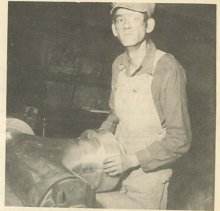
Bill Lynch was more than a little surprised when he looked up from his pattern work to find himself face to face with the camera. He was working on an aluminum pattern for hydrant bottoms.
