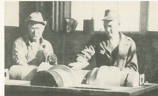
Buck Dempsey and Junior Wilcutt shown rigging a pattern for the jolter in the Special Foundry.
