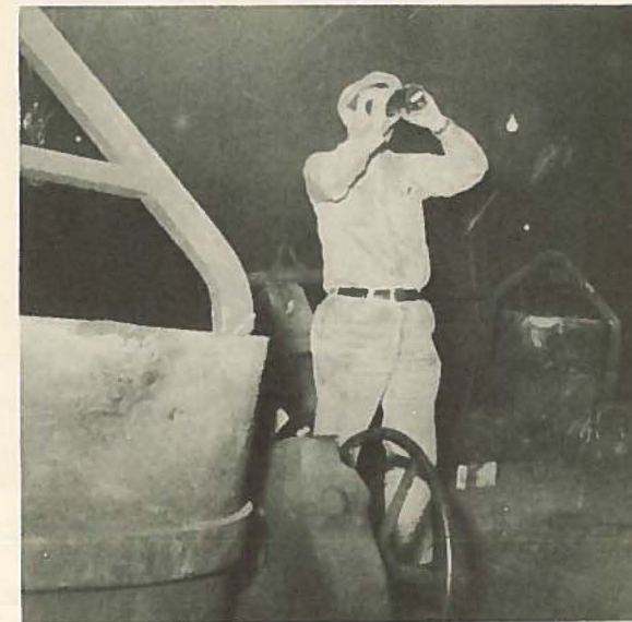
Ronnie Showman, assistant foreman, keeps close check on the iron heat with an optical pyrometer.
