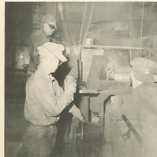
Dave Atchison (background) tips the mixing ladle to load a transfer ladle with molten iron for Bob McLandsborough (left) and Hugo Bracy.
