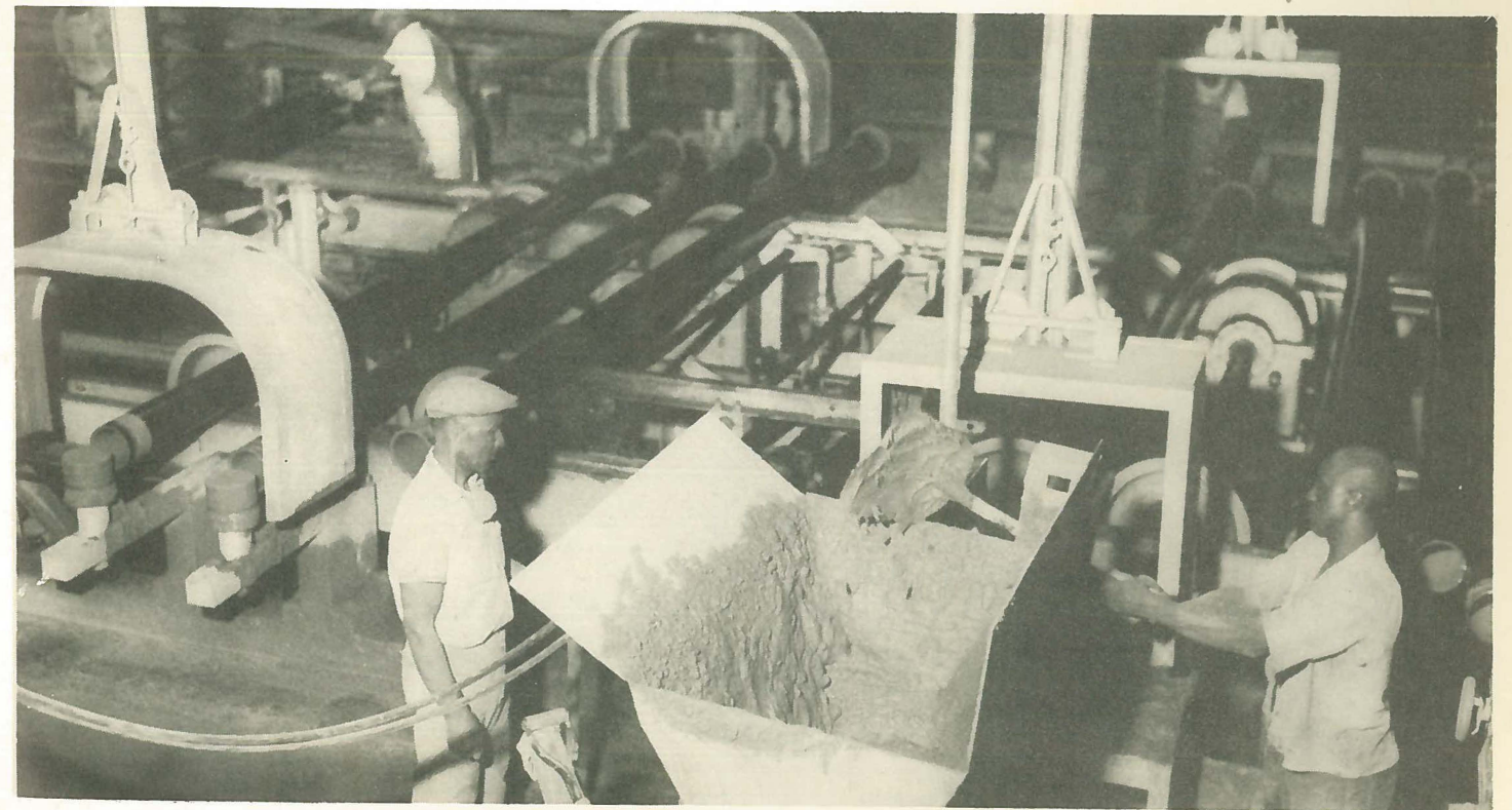
Johnnie Williams and Clarence Larkins are shown at the new pipe machine which automatically cement lines pipe.
