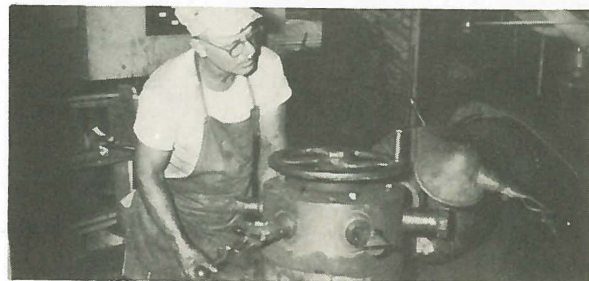
Tom Simms intently watches the machining of hydrant nozzle caps on his turret lathe. He recently transferred to this job from the small valve assembly.
