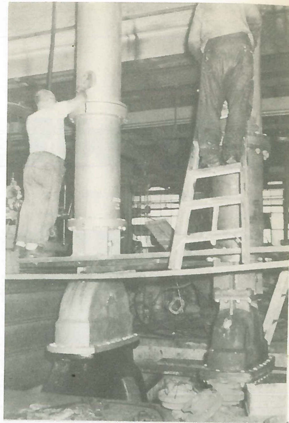
Valve mounter, Art Charbonneau on the right, puts the finishing touches on a cylinder valve while Harold Bornt begins the task of coating the other valve with asphaltum paint.
