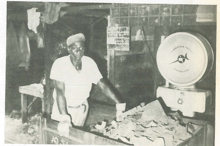
Osia Dansby weighs a load of scrap iron prior to charging the cupola with same.
