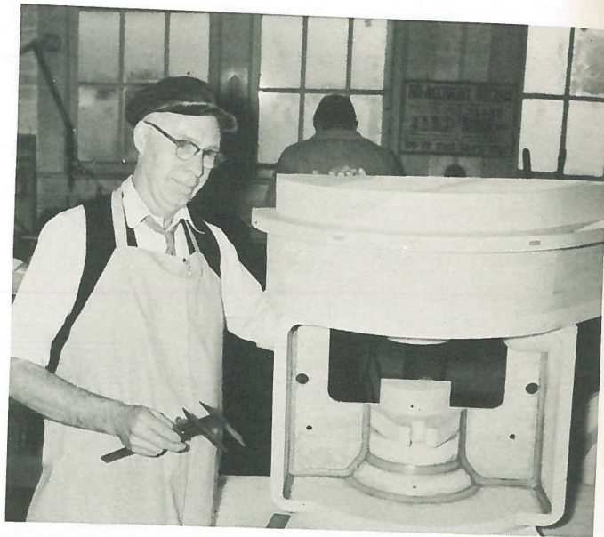
FRANK VAN DERWERKEN displays a pattern he is working on. FRANK has been with us for only a short time, but has proved to be a worthy addition to our Pattern Shop Crew. The pattern shown is for a 48" gear case.
