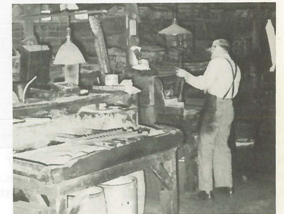
Curly Wise is shown filing the rough edges off a burner core.
