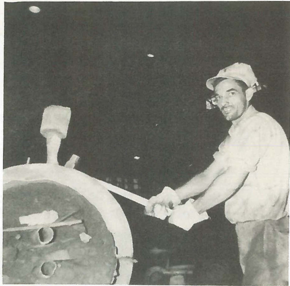
At left: James Stiers, knocking out a core in the Molding Floor Finish Department
