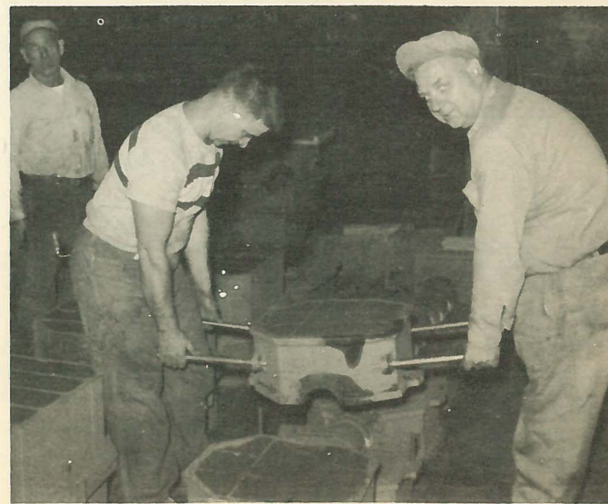
EDDIE LEMROW and JIMMY RYAN place the top section of a 4" body mold in place.
