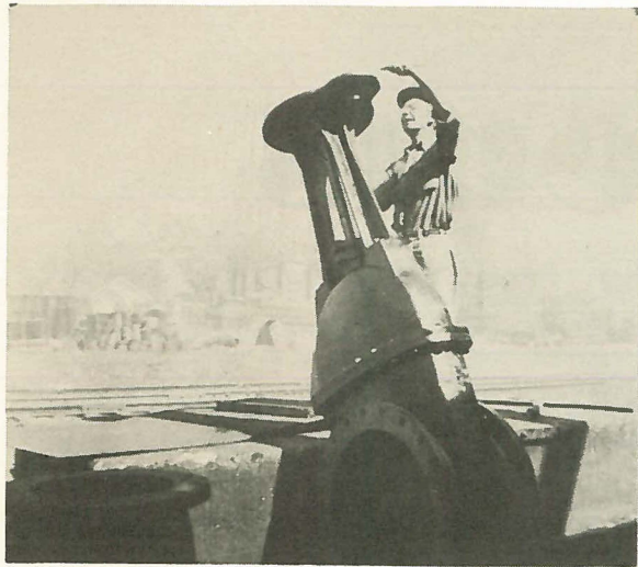
George Young takes a measurement on a 24" list 10 flanged valve with outside stem and yoke, grease case and handwheel. This is the first such valve made at Iowa.
