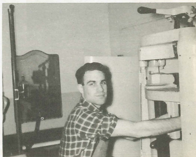
PETE inserts a test bar of cast iron into the tensile testing machine. This machine pulls the test bar apart and registers the pounds pull required to pull the bar apart.
