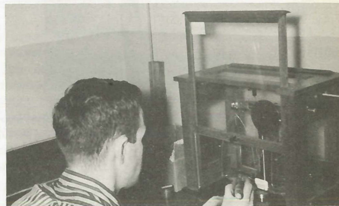
Cast iron filings are being weighed to a prescribed amount for use in the carbon determination test.
