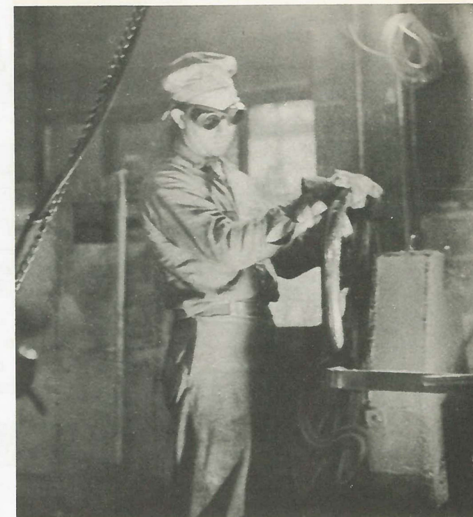
REX BARNHILL, peering through his protective glasses, is caught by the camera as he tips the mixing ladle in front of the cupola.
