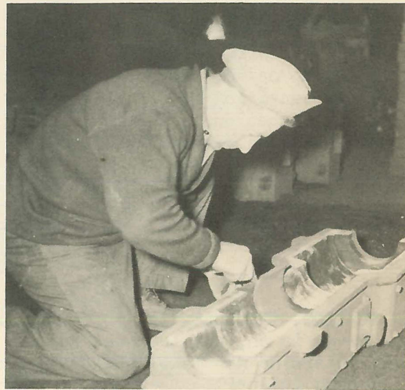
Peaches Montanari came to Eddy when the Clow regime got under way in 1945, and is here shown molding, with a valve box as the object of his affections.
