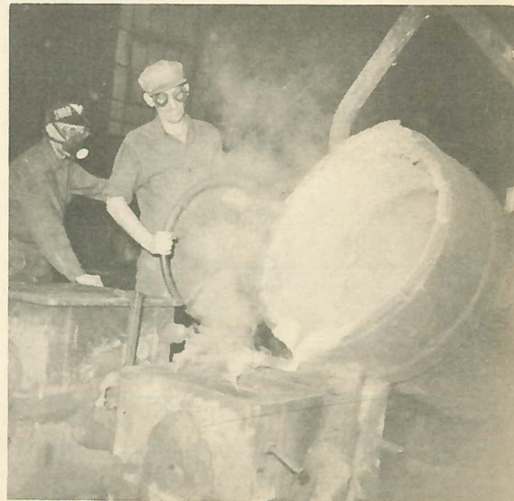
Tom Rees pouring off some of the smaller molds on the crane floor as Vess Earl in the background (with respirator) looks on. Despite the size of the mold he is pouring, Tom does the molding on all our largest castings.
