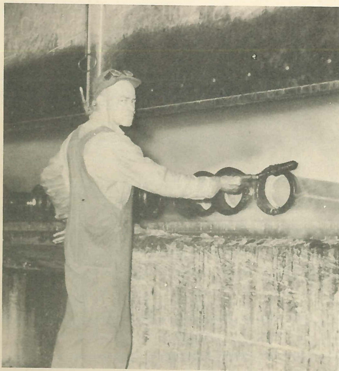
Roy Spruce, who works in the deLavaud Finishing Department is shown painting the end of a pipe.
