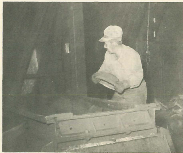
Bob Fisher on the foundry shakeout crew tosses a hydrant dome from the shaker screen.
