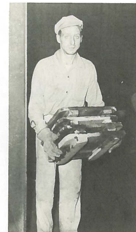
Ellis Miller stows bottom boards as he changes weights and jackets on a molding floor.
