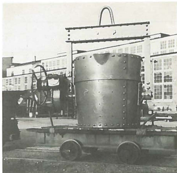
A new seven-ton ladle about to be made ready for use in the foundry.
