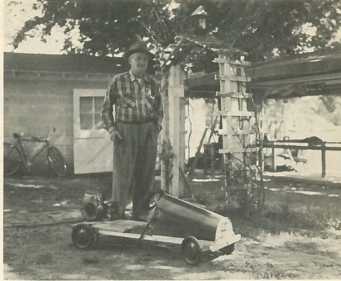
ABNER NELMS is shown with one of his midget automobiles. AB tells us these automobiles are equipped with a 2½ horse motor, and have a speed up to 18 miles per hour. They have a weight capacity of 150 pounds.
