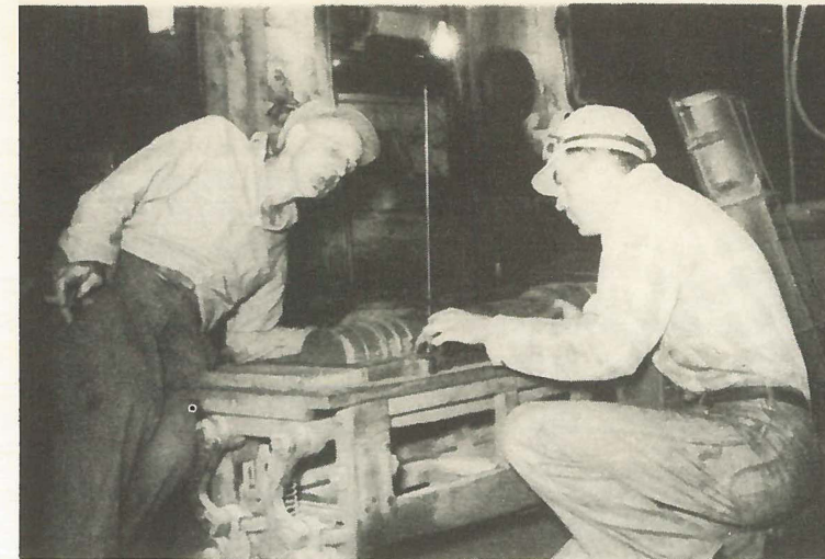
Bob Korns sights while Willard Donley gages up a valve box pattern.
