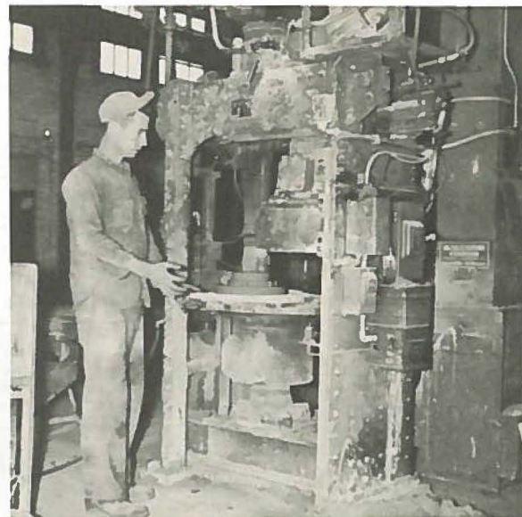
John Smith tends the new core blower.
