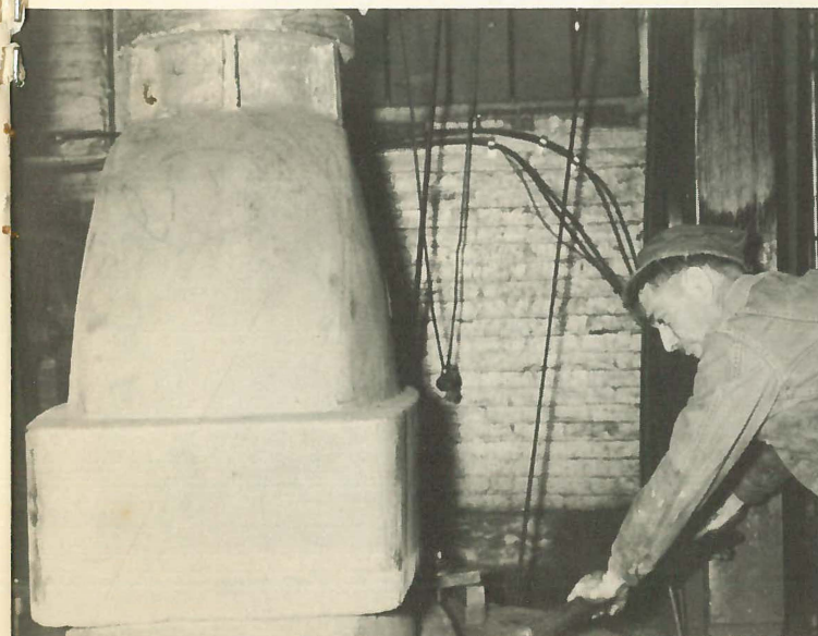
At left: GEORGE BOYER sets up a 48-inch body on the large boring mill.
