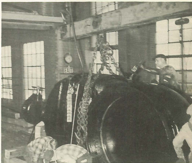
Here is a picture of the first 60-inch valve receiving a coat of paint just prior to its being loaded onto a transport truck that will carry it to the City of Buffalo. HAROLD BORNT, upper right, is our valve painter.
