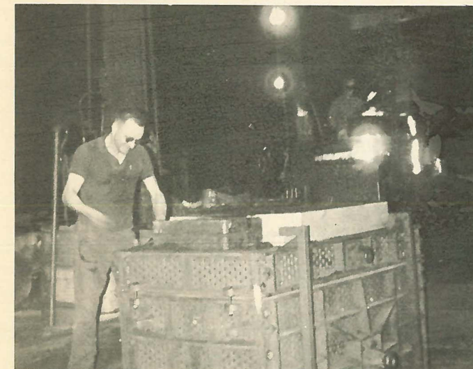
PAUL SHERMAN was caught putting the finishing touches to his first 36-inch valve case mold. In the right-hand background, REX BARNHILL can be seen behind the cupola spout.
