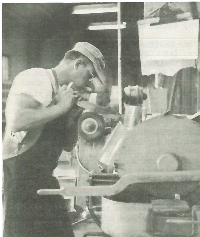
Part of the new brass foundry layout includes this abrasive cut-off unit operated by Lee Moffit of our machine shop.
