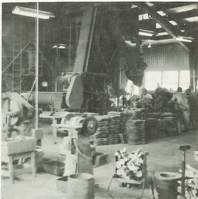
This is one of the views of the new Brass Foundry showing Bob Fisher operating the squeeze molding machine.
