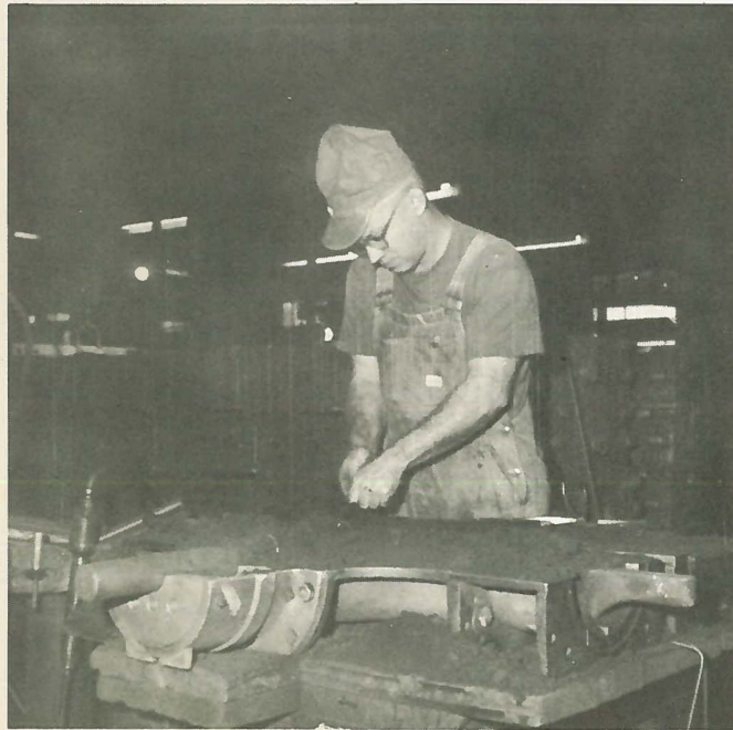
Looking into our iron foundry we found Bill Longcor busily engaged in making the green sand core for one of our hydrant bottoms.
