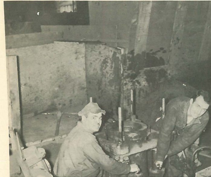
RALPH LOMBARDO on the left and JACK SCULLON make repairs on a molding machine in the Iron Foundry.
