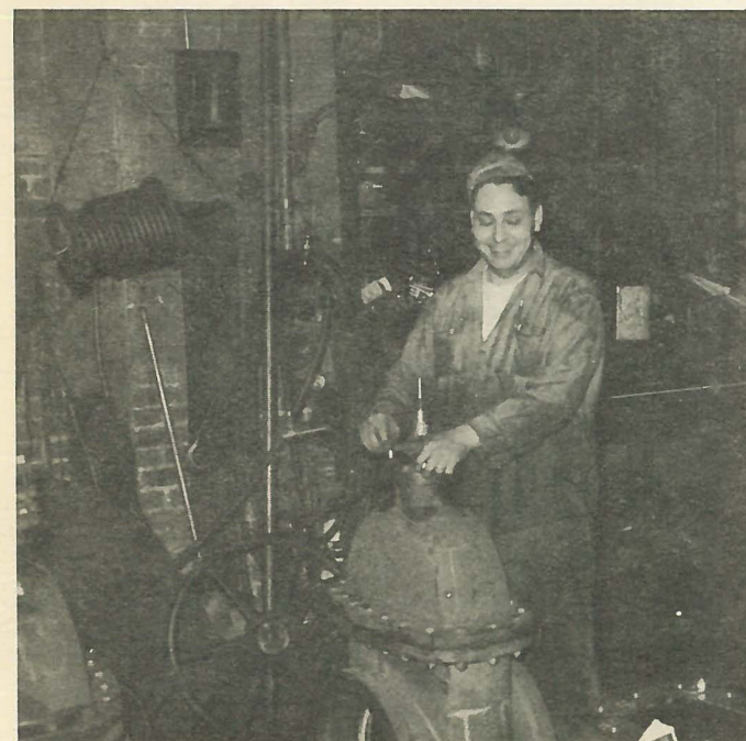
GERRY LAHUE slips a follower onto a 14" valve. GERRY mounts valves on our big valve mounting floor.
